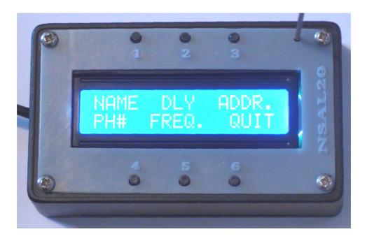
Your NAME, ADDRESS, and PHONE# can be changed using the buttons. It is NOT recommended that you change the preset DLY (Response Delay) or preset Frequency. Changing the frequency means you will no longer be able to communicate with the other NSAL units unless they also change the frequency. Changing the Response Delay could result in two or more NSAL units responding at the same time which could result in no proper response.
