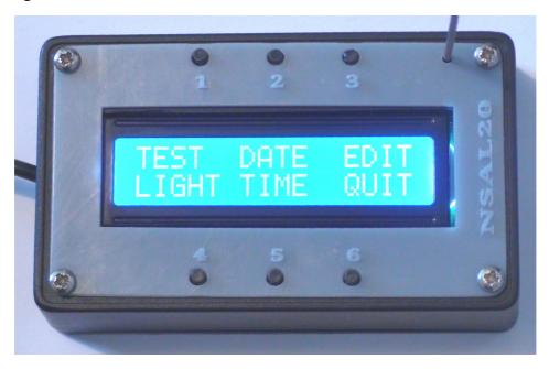
Pressing Button1 will result in a TEST signal being sent out to all the other NSAL20 units. All the units that have received the TEST signal will automatically send a response signal and not sound any alarms. This enables you to see who can and who cannot receive your emergency signals. The unit that sent the TEST signal will display the information about which neighbors received the TEST signal and responded.
